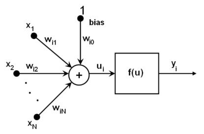
In other words, given the outputs  $x_i$  of the layer n , the outputs  $y_i$  of the layer n + 1 are computed as:
